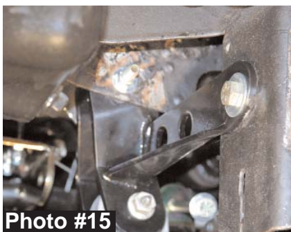
REAR mounting point on passenger side diff tube.
